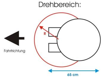
When choosing the mounting location, keep in mind, that the cables to the external unit are 6 m long and that the external unit must have sufficient free space to turn.
